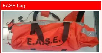
A dedicated EASE bag is stowed on all operational appliances. The design of the bag allows a BA set to be placed within the bag with the female couplings and bodyguard unit protruding from one end. Carrying handles are also provided. A bodyguard key and protective caps are also provided.
